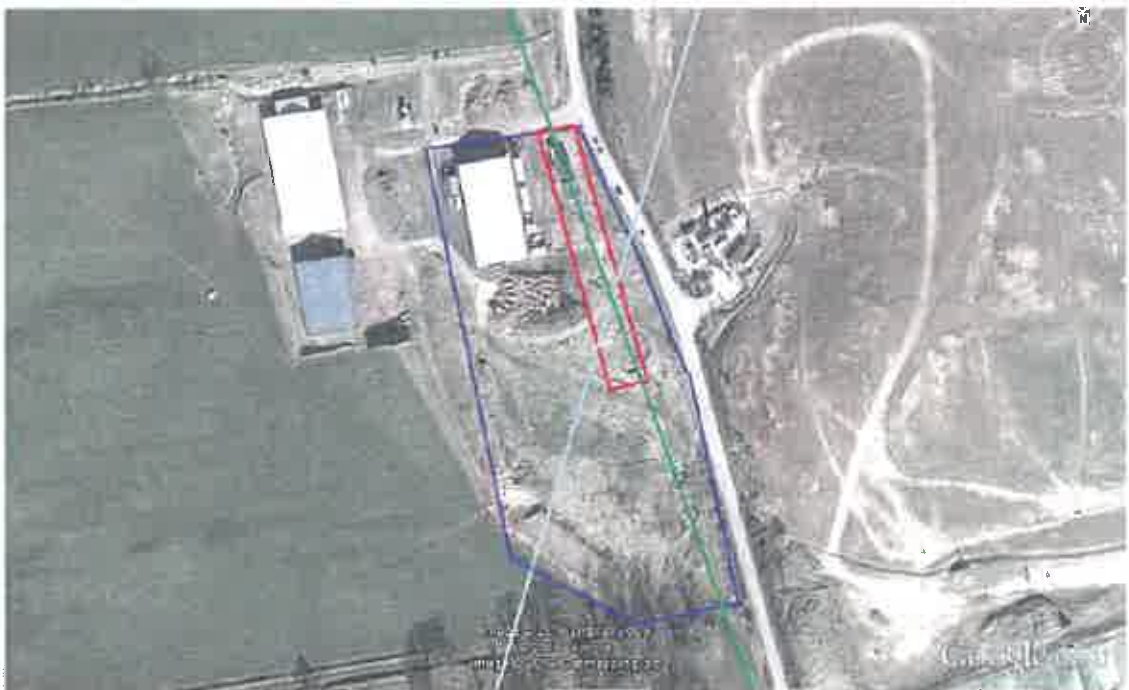
Figure 2: Aerial of site showing boundary (red) overhead power line (pale blue) and gas pipe (green)
